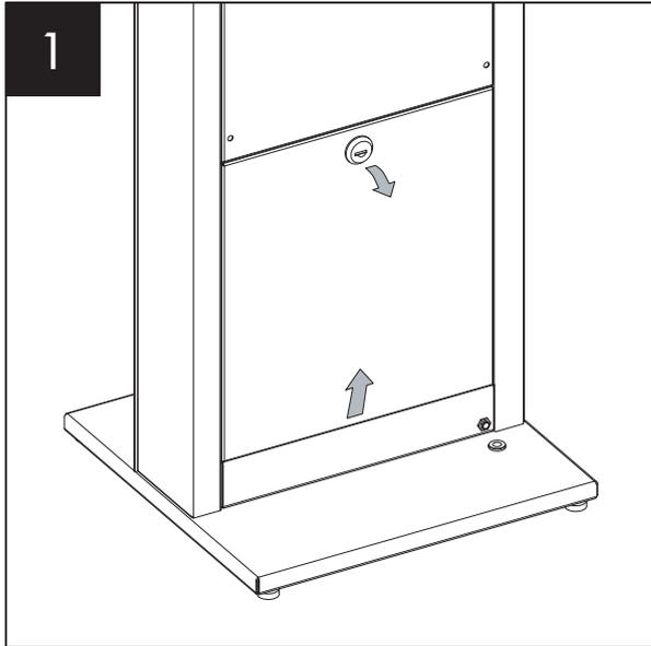
Remove the rear access cover located at the rear of the unit by unlocking the catch and then lifting up the cover.
