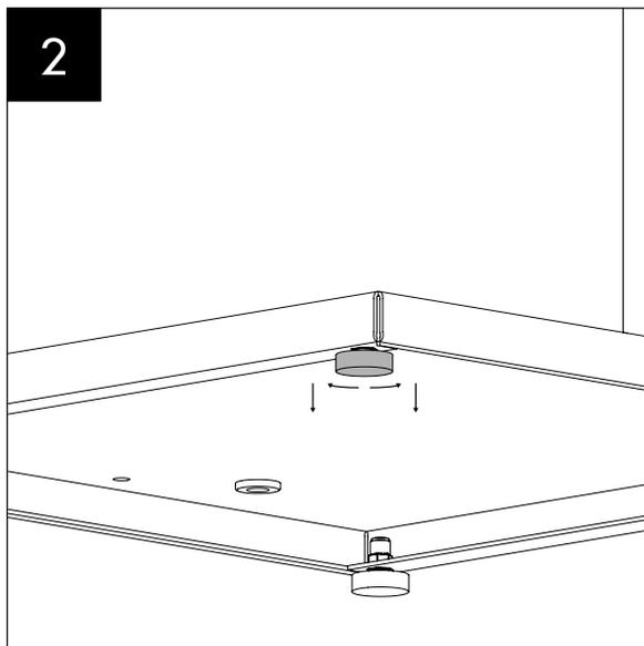
The cabinet can then be levelled using the 4 adjustable feet on the underside of the base.
