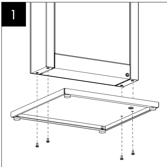
Lay down the cabinet on its side on a soft surface to avoid scratching. Fit the base to the underside of the unit and fix with the 4 screws provided.
