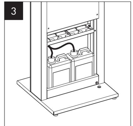
Insert the hoses into the containers ensuring they are pushed to the bottom.
