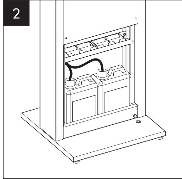
Remove silicone hoses and either replace the sanitiser containers or top up as required. Insert the hoses back into the bottom of the containers.
