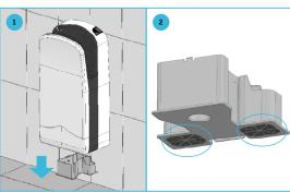
Air Filters: To be checked often and cleaned if necessary.
